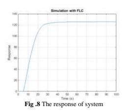
The system response shows that the Controller designed for the steam boiler offers a high performance with low overshoot and short settling time.
